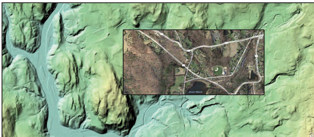
Lidar shaded relief of the Moodus, CT area (Salmon River on left). A portion of a terrain map is superimposed to highlight the fine detail of the lidar image.
