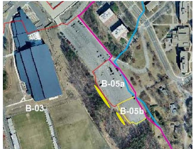
Figure 1. Drainage areas to two proposed bioretention cells.
