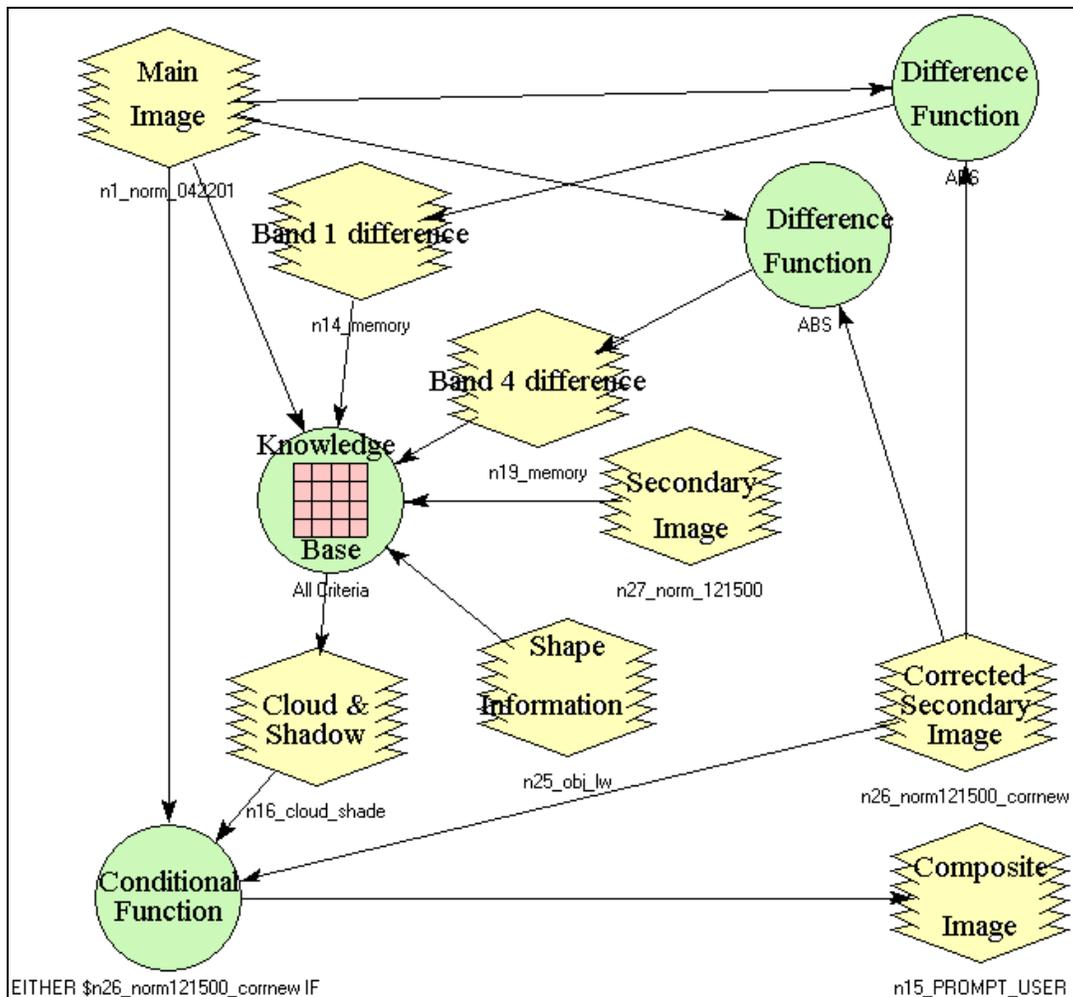
Figure 4. Flowchart of cloud and shadow reduction in Imagine Spatial Modeler format
