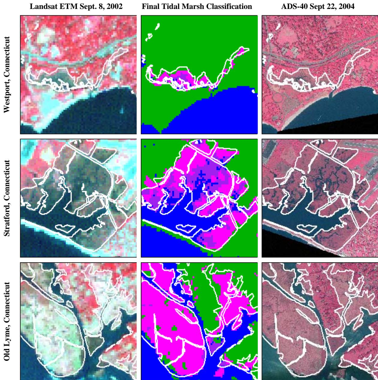
**Figure 8.** Results of the final integrated tidal marsh classification for selected areas along the Connecticut coast compared with the Landsat ETM image used for classification and a high spatial resolution ADS-40 image. The white outlines represent tidal marshes delineated from aerial imagery by Connecticut Department of Environmental Protection personnel. In the classification, green represents upland, blue is water, magenta is high marsh, and purple is low marsh.
