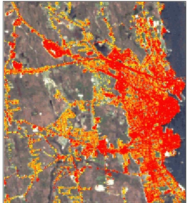
**Figure 2A.** IMAGINE Subpixel Classifier overlay image for impervious surfaces.
