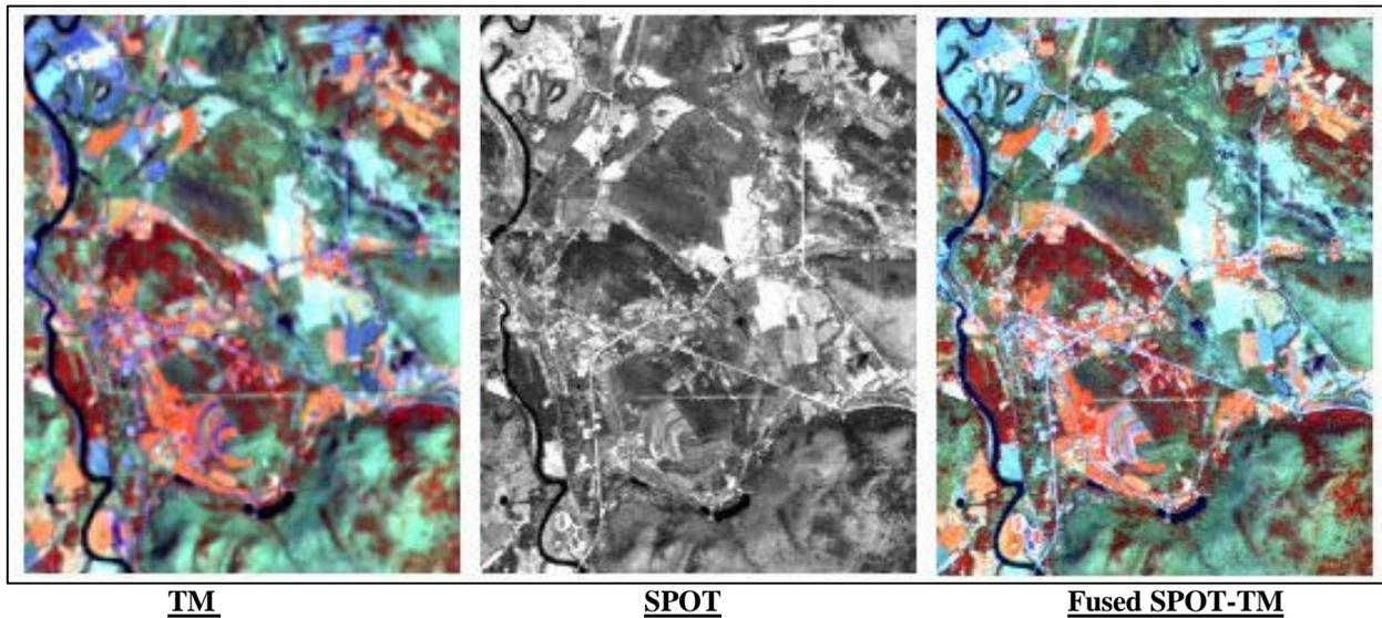
**Figure 3.** Example of 30 meter TM data (Bands 4, 5, 3) fused with 10 meter SPOT Panchromatic data.
